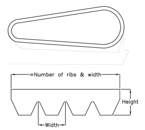
$\begin{array}{ll} \text{Datum Llength} = 2743 \\ \text{Height} &= 9.5 \\ \text{Number of ribs} = 20 \\ \text{Pitch} &= 4.7 \end{array}$
